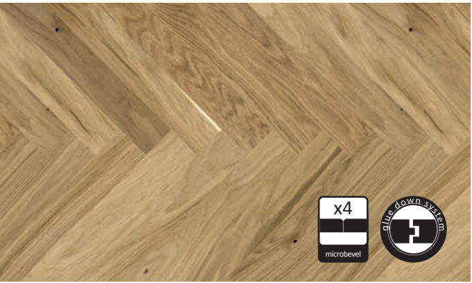
5906737985540 660 x 110 x 14 mm OAK CARAMEL CLASSIC HERRINGBONE 110 brushed, 4 side micro bevelled, matt lacquered 刷面， 4面微斜切，哑光漆面
